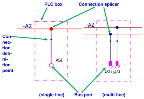
Use a symbol with fitting connection number for the multi-line representation (see chapter Displaying Bus Ports in Multi-line in Eplan Help).
