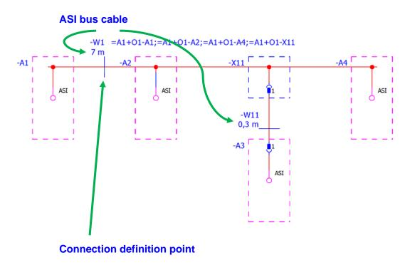
3. The display of the list of the connection splicers passed through can also be carried out line-oriented (under each other) by using an alignment box.
